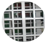
Bisection of the inner trommel approx. 75 x 75 mm
