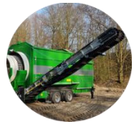
Extended conveyor belt for middle fraction
