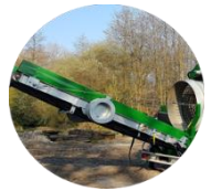
Extended conveyor for coarse fraction
